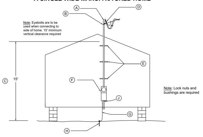
Note: This diagram is to be used as a guide only. Some installations may vary. All installations must meet NEC, NESC, and BRIGHTRIDGE Requirements.
